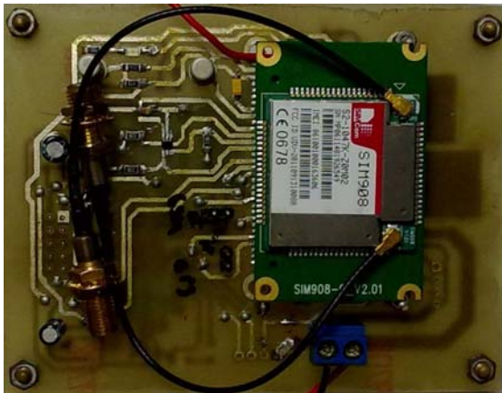
Figure 5a. Top side of the GPS vehicle tracking with the SIM908 module shown on top of it
