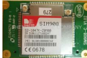
Figure 2b. Top view of SIMCOM908 module with I-Pex antenna connector.
