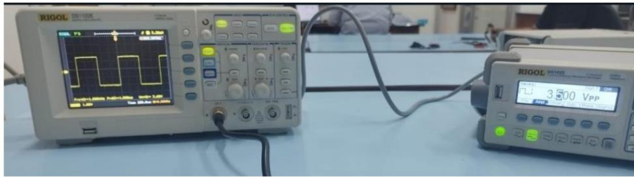
Figure 7. A square wave is generated by a signal generator and observed by using an oscilloscope
