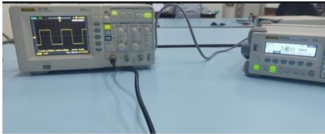
FIGURE 7. A square wave is generated by a signal generator and observed by using an oscilloscope.
