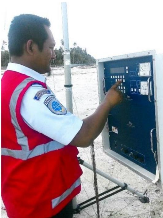
**Gambar 6** Setting Transmitter NDB Portable
