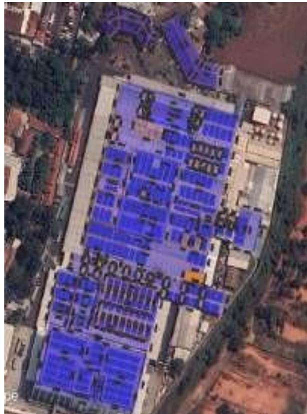
Figure 2 Layout Of Solar Panel Application In PTADF
