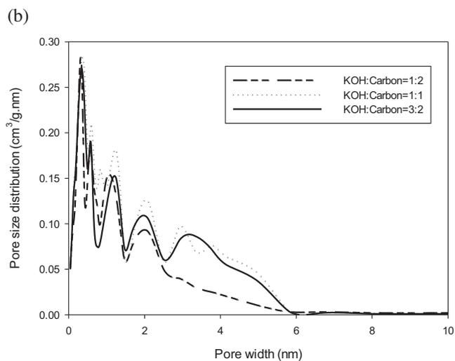
**Fig. 2.** Pore structure of the carbon microsphere and its activated forms (a) nitrogen adsorption isotherms and (b) DFT pore size distribution of activated carbons.
