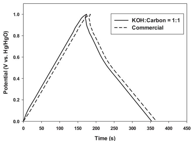
**Fig. 4.** Galvanostatic charge and discharge of carbon electrode and commercial activated carbon electrode at a current density of 1 A/g.
