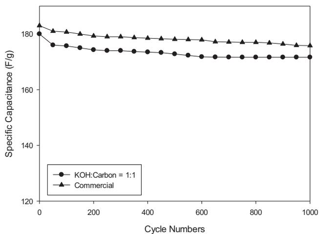
**Fig. 3.** Cycling stability performance curves for activated carbon microsphere with impregnation ratio 1:1 and commercial electrode.
