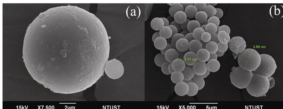
**Fig. 1.** SEM images of carbon microsphere synthesized at temperature of 180 °C and 10 h.
