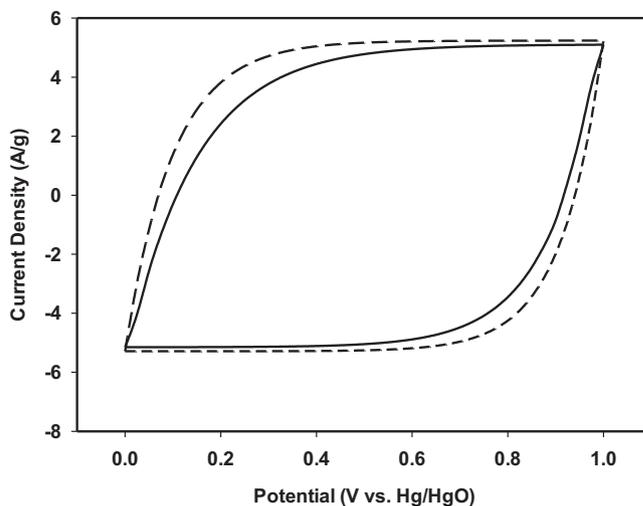
**Fig. 5.** Cyclic voltammograms of activated carbon microsphere with impregnation ratio 1:1 (solid line) and commercial activated carbon electrode (dash line).
