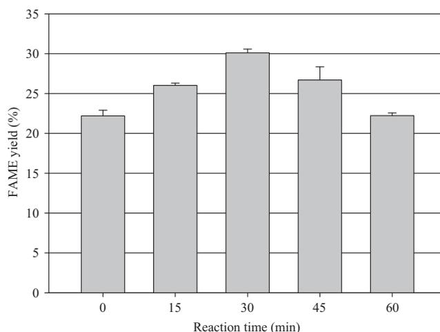
Fig. 6. Effect of reaction time on FAME yield at  $250^\circ\text{C}$ , a solvent (methanol/AA, 15% acetic acid) to dry sludge ratio of  $5 \text{ mL g}^{-1}$ .
