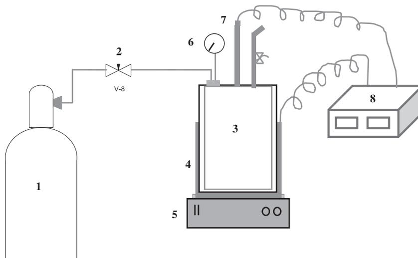
**Fig. 1.** Layout of equipments for in situ transesterification of activated sludge. [1] Nitrogen cylinder, [2] needle valve, [3] reactor, [4] heater, [5] magnetic stirrer, [6] pressure gauge, [7] thermo couple, [8] controller.
