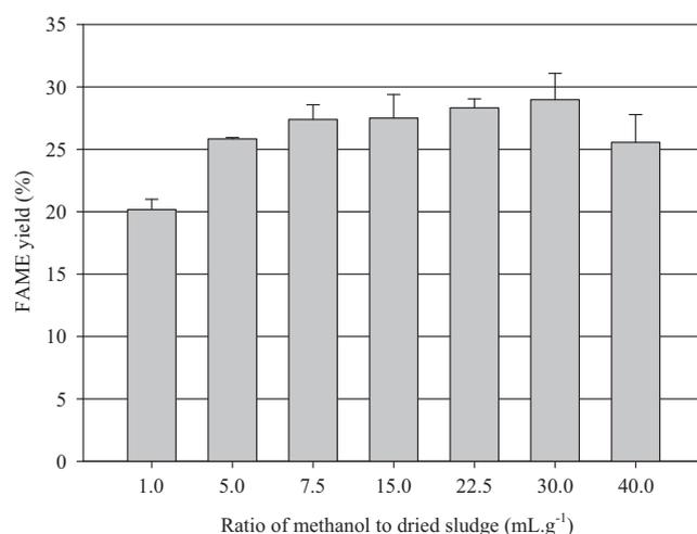
Fig. 4. Effect of methanol to dry sludge ratio on FAME yield. Reaction temperature = 250 °C, reaction time = 120 min.
