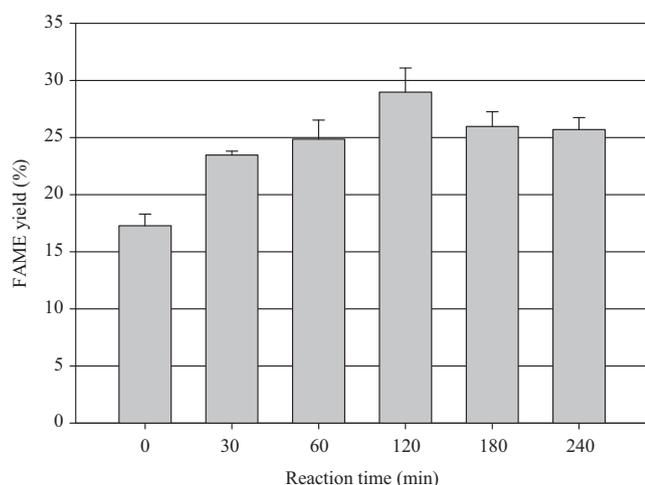
Fig. 3. Effect of reaction time on FAME yield at 250 °C with a methanol to dry sludge ratio of 30 mL g<sup>-1</sup>.
