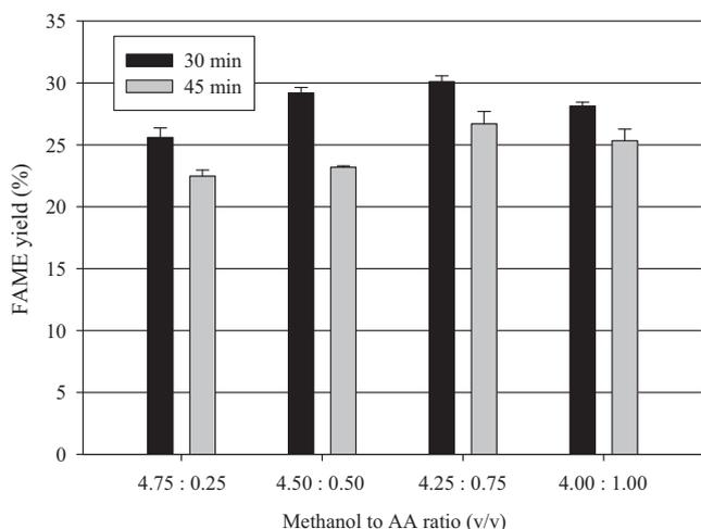
Fig. 5. Effect of AA loading on FAME yield at  $250^\circ\text{C}$ , a solvent (methanol/AA) to dry sludge ratio of  $5 \text{ mL g}^{-1}$  and reaction time of 30 and 40 min.
