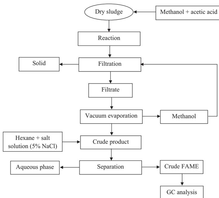
**Fig. 2.** Flowchart of biodiesel production from dried sludge.
