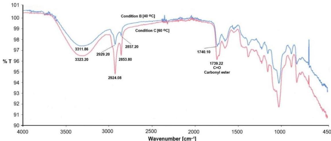
Figure 3: CA-LBG infrared spectra at 40°C and 60°C
