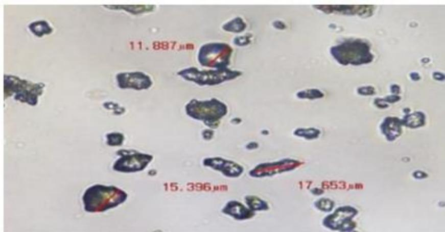
**Figure 1.** Microscopic picture of polyethylene particles that have been filtered to a size less than 20  $\mu\text{m}$  using the FCT Z100 miller machine.
