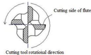
**Fig. 2** Cutting Tool Cross Section [3]
