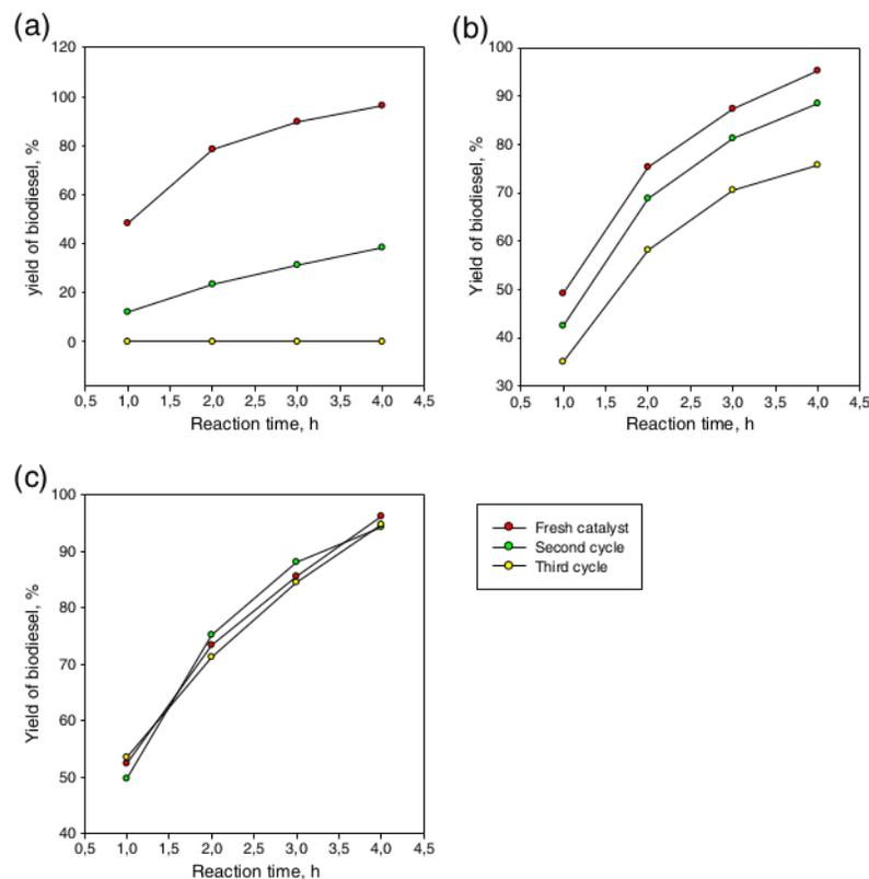
**Figure 5** The yield of biodiesel at different spent catalyst treatments under cycle reaction conditions. (a) Untreated spent catalyst, (b) washing of spent catalyst with organic solvent, and (c) re-calcination of spent catalyst.
