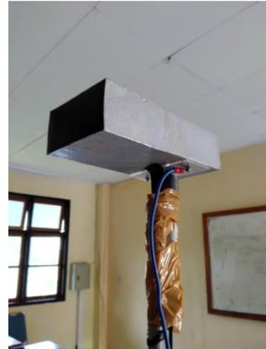
Figure 3. Horn Antenna
