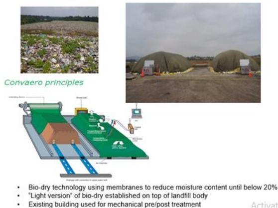
Fig.3. Bio-drying method (*convaero* system)
