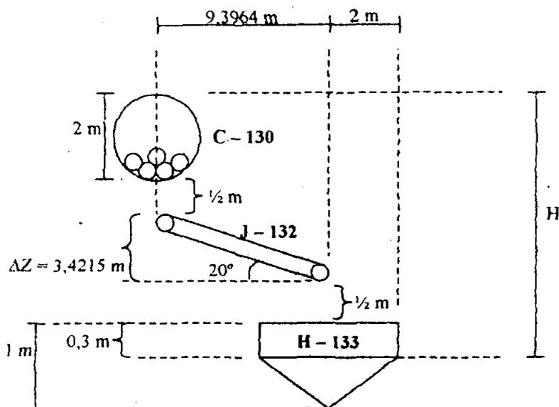
$H$  = tinggi Tumbling Mill C – 130 + jarak Tumbling Mill ke Belt Conveyor J – 132 + tinggi Belt Conveyor J – 132 + jarak Belt Conveyor ke Screen H – 133 + tinggi Screen
