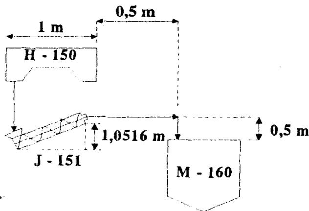
$$\text{Panjang Screw Conveyor J - 151} = \sqrt{5,0904^2 + 4,9212^2} \text{ ft} = 7,0803 \text{ ft} \approx 10 \text{ ft}$$
