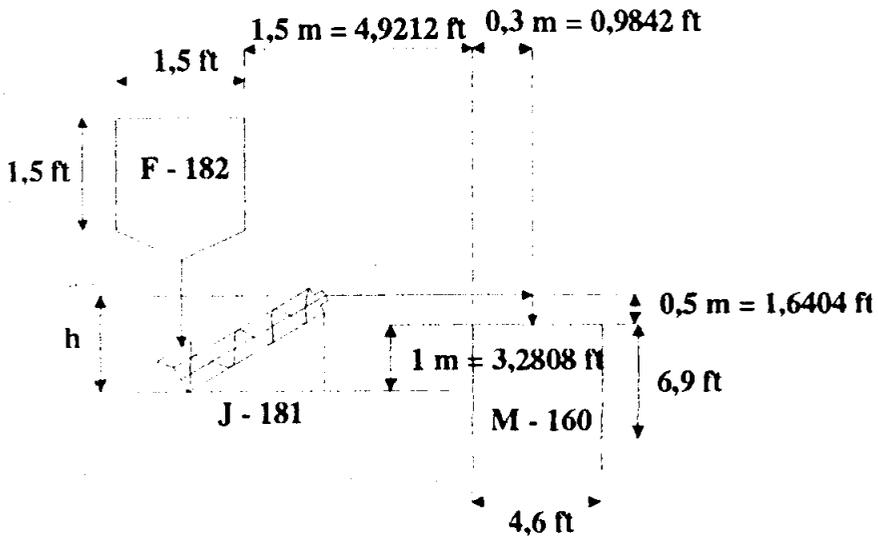
$$\text{Panjang Screw Conveyor J - 181} = \sqrt{6,6554^2 + 4,9212^2} \text{ ft} = 8,2773 \text{ ft} \approx 10 \text{ ft}$$
