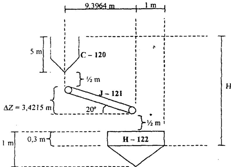
H = tinggi Jaw Crusher C – 120 + jarak Jaw Crusher ke Belt Conveyor J – 121
