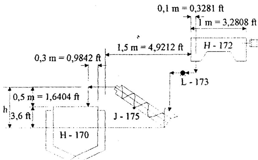
$$\text{Panjang Screw Conveyor J - 175} = \sqrt{6,2335^2 + 5,2404^2} \text{ ft} = 8,1436 \text{ ft} \approx 10 \text{ ft}$$
