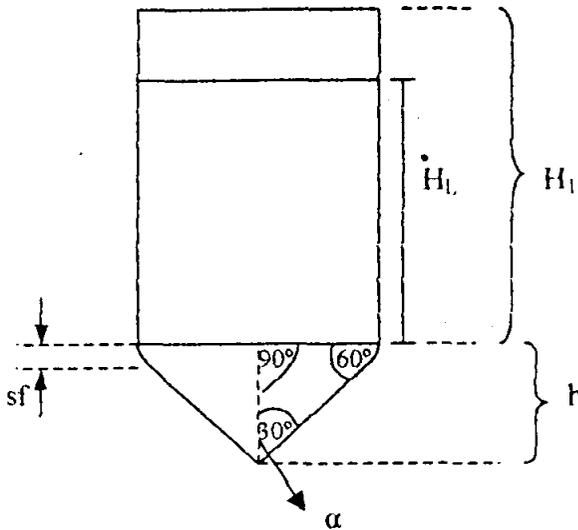
$$\text{Tinggi konis (h)} = \frac{0,5 \cdot D}{\tan 60^\circ} = \frac{0,5 \cdot 22 \text{ ft}}{\tan 60^\circ} = 6,3447 \text{ ft} = 1,9339 \text{ m}$$
