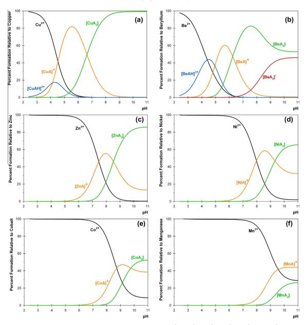
Fig. 6. Species distributions for binary system of 2-aminophenol (A) and the metal(II) ion: (a)  $Cu^{2+}$ ; (b)  $Be^{2+}$ ; (c)  $Zn^{2+}$ ; (d)  $Ni^{2+}$ ; (e)  $Co^{2+}$ ; and (f)  $Mn^{2+}$ ; at a 1:2.5 metal to ligand ratio,  $T = 37 \pm 0.1$  °C and I = 0.15 mol dm<sup>-3</sup> NaCl.
