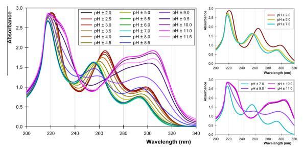
Fig. 4. UV–Vis spectra of 3,4-dihydroxybenzoic acid (D), where [D] = 0.001 mol dm<sup>-3</sup>,  $T = 37 \pm 0.1$  °C, I = 0.15 mol dm<sup>-3</sup> NaCl.
