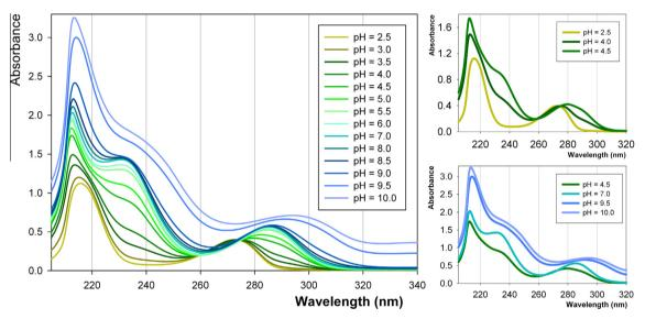
Fig. 3. UV-Vis spectra of 2-aminophenol (A), where [A] = 0.001 mol dm<sup>-3</sup>,  $T = 37 \pm 0.1$  °C, I = 0.15 mol dm<sup>-3</sup> NaCl.
