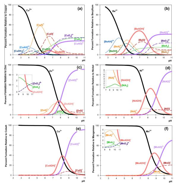
Fig. 8. Species distribution for ternary systems involving: (a)  $Cu^{2+}$ , (b)  $Be^{2+}$ , (c)  $Zn^{2+}$ , (d)  $Ni^{2+}$ , (e)  $Co^{2+}$  and (f)  $Mn^{2+}$  at a 1:1 metal to ligand ratio,  $T = 37 \pm 0.1$  °C and I = 0.15 mol dm<sup>-3</sup> NaCl.
