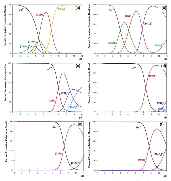
Fig. 7. Species distributions for the binary systems of 3,4-dihydroxybenzoic acid (D) and the metal(II) ions: (a)  $Cu^{2+}$ ; (b)  $Be^{2+}$ ; (c)  $Zn^{2+}$ ; (d)  $Ni^{2+}$ ; (e)  $Co^{2+}$  and (f)  $Mn^{2+}$ ; at a 1:2.5 metal to ligand ratio,  $T = 37 \pm 0.1$  °C and I = 0.15 mol dm<sup>-3</sup> NaCl.
