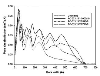
**Fig. 2** Pore size distributions of untreated and modified carbons with medium level of software regularization.
