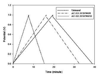
Fig. 5 Galvanostatic charge-discharge curves of untreated and modified carbon electrodes.
