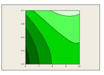
(a) (b) Figure 1. Tensile strength of biodegradable film as the effect of gathotanand tapioca concentration (a) surface plot (b) contour plot.
