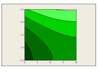
(a) (b) Figure 2. Tensile strength of film as the effect of glycerol and gathotan flour concentration (a) surfaceplot, (b) contourplot
