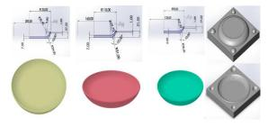
**Gambar 6.** 3D model gambar desain piring, master core dan cavity piring *couple tableware* motif Kawung
