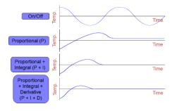
**Gambar 4**. Gambaran hasil Actual Point : On-Off vs P vs PI vs PID terhadap Set Point
