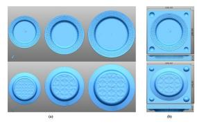
**Gambar 5.** 3D model piring *tableware* motif Kawung: (a) desain dining plate, (b) desain master *core* dan *cavity*
