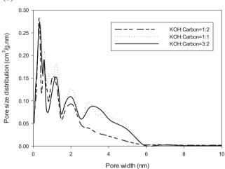
**Fig. 2.** Pore structure of the carbon microsphere and its activated forms (a) nitrogen adsorption isotherms and (b) DFT pore size distribution of activated carbons.
