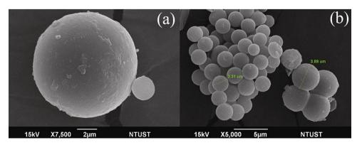
Fig. 1. SEM images of carbon microsphere synthesized at temperature of 180 °C and 10 h.
