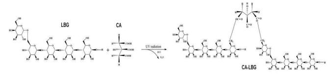
Figure 1: CA-LBG esterification mechanism
