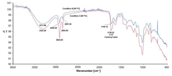
Figure 3: CA-LBG infrared spectra at 40°C and 60°C
