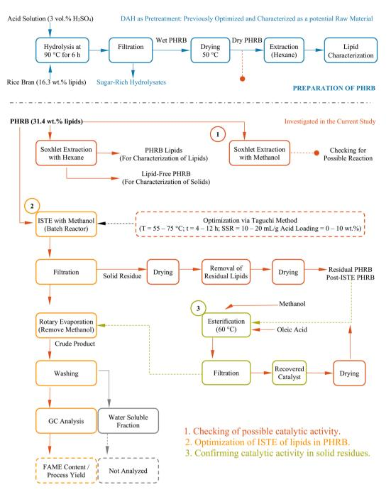
Fig. 1. Schematic flow diagram of producing PHRB, ISTE of lipids in PHRB and subsequent use of post-ISTE PHRB "This figure is to be printed in black and white".
