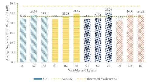
**Fig. 3.** Response graph of the-higher-the-better S/N ratios of FAME yield (S/N<sub>ave</sub> = 23.31). A: temperature (55, 65, 75 °C); B: solvent-to- solid ratio (SSR: 10, 15, 20 mL/g); C: time (4, 8, 12 h); D:  $H_2SO_4$  (0, 5 10 wt% relative to the solids). "This figure is to be printed in black and white".
