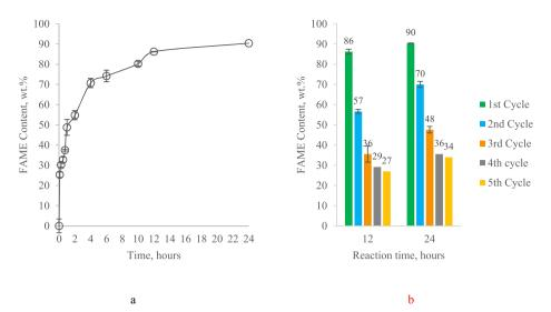
Fig. 5. Esterification of oleic acid with methanol (1st Cycle) at a solvent-to-oil ratio of 20 mol/mol for 24 h at 60 °C with constant stirring at 200 rpm (a) and reusability of PHRB residues after ISTE as catalyst (b). "This figure is to be printed in black and white".
