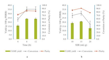
Fig. 2. The catalytic activity of PHRB during ISTE without the addition of catalyst for the reactions carried out in a Soxhlet extractor with an SSR of  $\sim$ 17 mL/g and under open reflux for 8 h (a) and in a batch reactor with different SSR of 10, 15, and 20 mL/g at 75 °C, for 8 h with constant stirring at 200 rpm (b). "This figure is to be printed in black and white".
