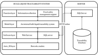
Fig. 2. The architecture of the bulk-liquid traceability system.
