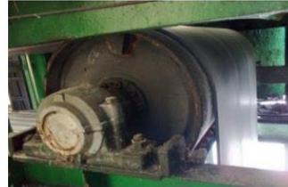
Gambar 4.5. *Bend Pulley*
