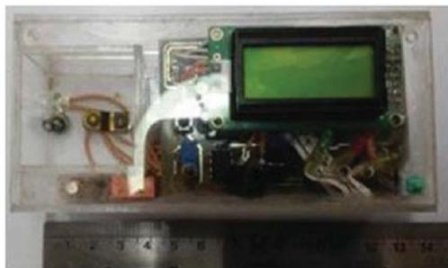
**Fig. 32.6** **a** Top circuit board with microcontroller.
