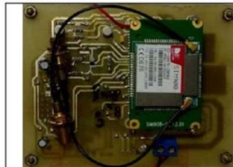
Figure-5a. Top side of the GPS vehicle tracking with the SIM908 module shown on top of it.
