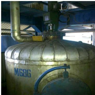
Gambar 7.2. *Degumming Process Tank (M-686)*
