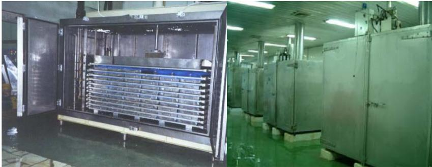
Gambar 7.3. *Contact Plate Freezer*
